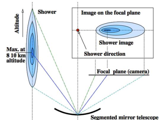
Imaging of a  $\gamma$ -ray initiated e.m. shower by a telescope. Image taken from [Völk and Bernlöhr \(2009\)](#)
