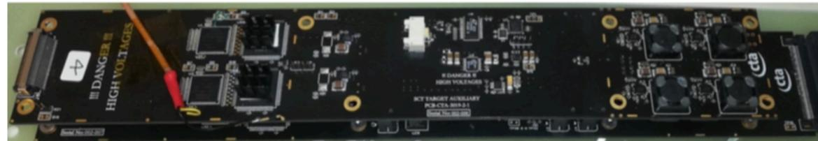
Figure 5. (top) Sketch of the upgraded camera FEE module, the Auxiliary and Primary boards are shown on top and bottom, respectively. Both boards have been logically divided into an analog and digital/power sections. (bottom) Picture of the prototype FEE module currently under test.
